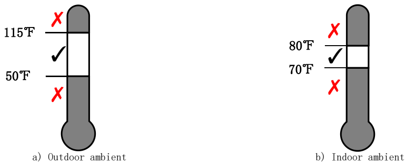
Fig 13-2 Temperature limit for AUTO charge mode
